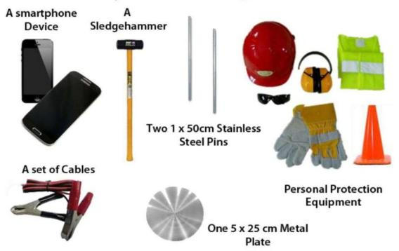
For our electro-seismics mapping work, we used the following equipment:
